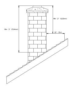
FIGURE 2.2 Minimum Height of the Chimney
